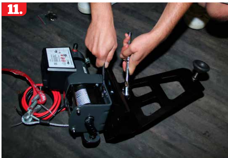
10. At this point, the center anchor and winch mounting bracket were bolted together, and the rubber stop was adjusted to our bulkhead. A plastic knob attaches to the front for easy adjustment.
