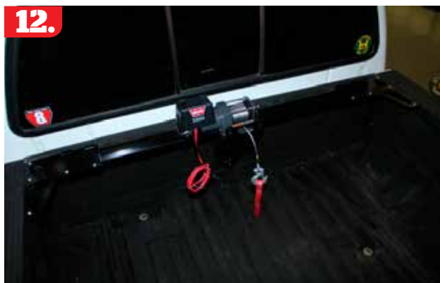
11. Now the Warn 2000 winch could be bolted to the mount. This will remain as one unit that can be removed or replaced in seconds.
