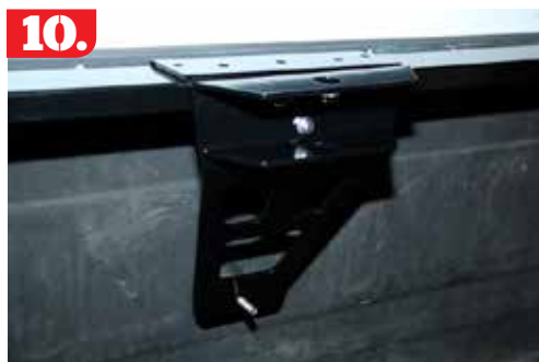
10. At this point, the center anchor and winch mounting bracket were bolted together, and the rubber stop was adjusted to our bulkhead. A plastic knob attaches to the front for easy adjustment.
