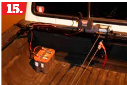
12. The winch assembly was set in place and locked down with the supplied knobs. It was now time to hook up a power supply.
